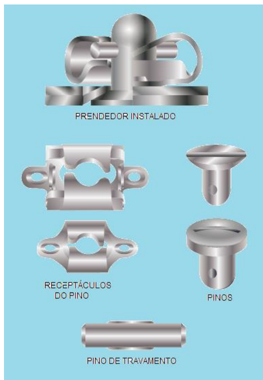
Fonte: FAA - Federal Aviation Administration - Mechanic Training Handbook Figura 6-20 Prendedor Airloc.
