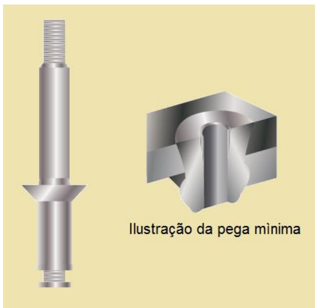
Fonte: FAA - Federal Aviation Administration - Mechanic Training Handbook Figura 6-39 Rebite "Cherry-lock" com bulbo.
