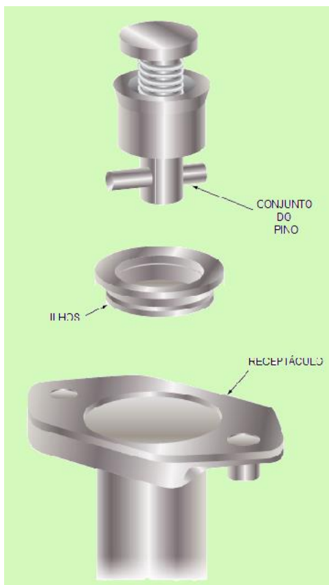
Fonte: FAA - Federal Aviation Administration - Mechanic Training Handbook Figura 6-19 Prendedor Camloc.
